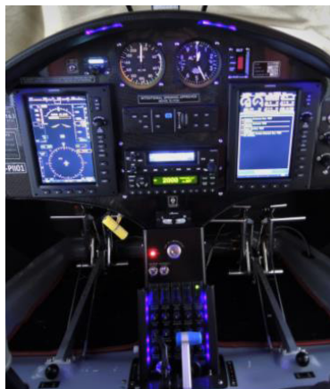
Figure 3 Glare-shield and breakers UV-LED lights
