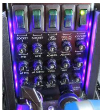
Figure 6 Circuit breakers UV-LED lights
