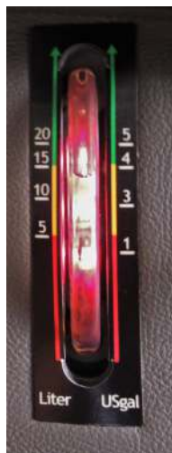
Figure 5 Fuel tank level LED lights
