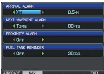
Nav Alarms (Split-Screen)
