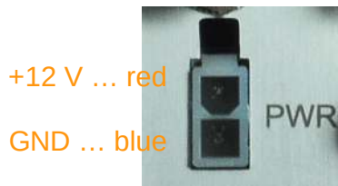
Figure 9: Pins of the power connector.
