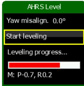
Figure 14: Illustration of AHRS levelling procedure.
