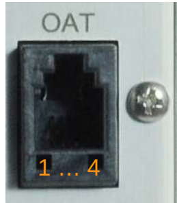
Figure 10: Pins of the OAT connector.
